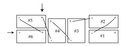
Two 6-volt batteries for 12 volts. Two 8-volt batteries for 16 volts.
