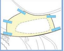
3.Use a marker or other marking device to trace the inside contour of the template.
