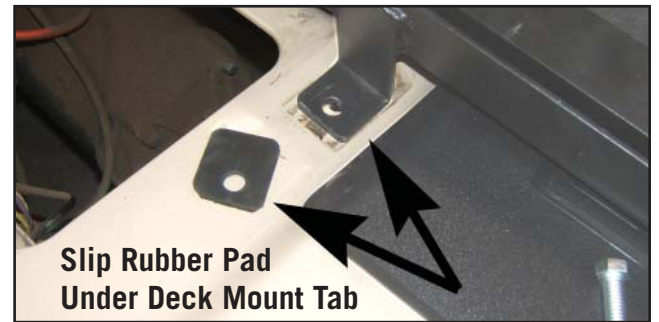
Fig. 7 - Rubber Pad Installation
