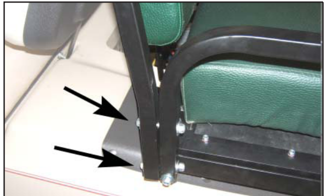
Fig. 14 - Install Top Supports
