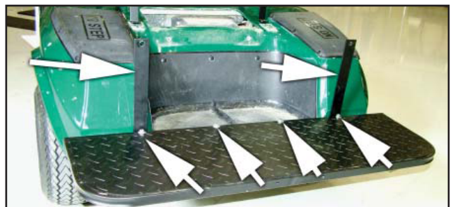
Fig. 4 - Install Rear Foot Rest Assembly
