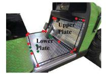
In the above picture (EZ-GO) notice the red dots represent recommended placement of the rivets. The green dots represent areas' you do not want to drill. For your Club Car or Yamaha lay out a similar pattern to aid in the correct spot for drilling.
