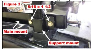
Picture is of driver side and looking from front of the car
