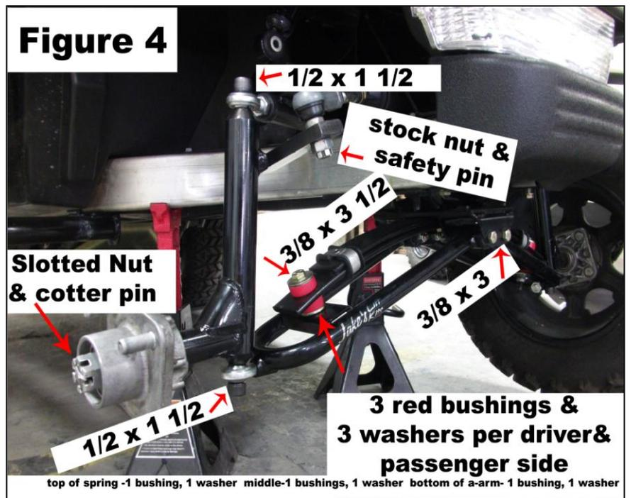
13. Using the supplied 1/2 x 1 1/2 socket head bolts mount the spindles to the upper and lower a-arms as shown in Figure 4. **NOTE: The spindles are side specific. Mount to the a-arms with the steering arm of the spindle towards the front of the cart.**
