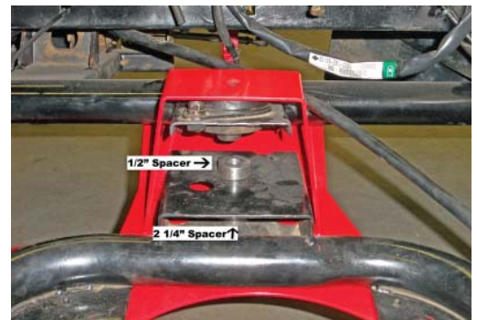
The remaining 1/2" spacer goes between the skid plate & stock front swing arm mount.
