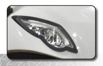
Align Tail Light template to the body as shown using the template notes for proper placement. Use a marking pen to trace the cut out. Drill a pilot hole as a starting point, then use a rotary cutting tool to cut out the tail light. Be sure to cut to the inside of the marked line. Use sandpaper to smooth edges.
