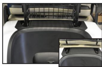
Place front main brackets into golf cart where factory basket was removed. Install hardware using retained hardware. Strut mounting tabs should be on the outside of the cart.
