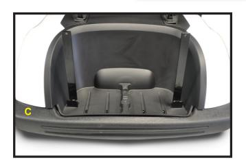
C) Attach bagwell bracket using retained hardware.
