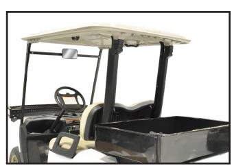
Attach cargo box using 10mm x 30mm hex head bolts. Once all bolts are in place, tighten all hardware.
