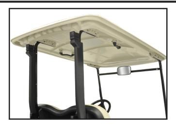
Remove hardware from gutters and retain. Remove gutters by sliding them upward.
