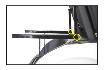
Attach cargo box bracket to bagwell bracket using 10mm x 25mm hardware, hand tighten.
