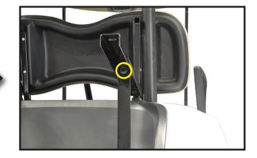
Reattach canopy using retained hardware from step 1.
