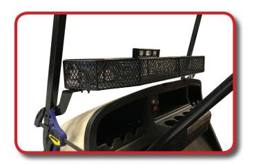
Drill hole through strut and secure using supplied 8mmx40mm bolts, washers and nuts.
