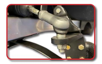
Attach the factory front wheel hub to the new Spindle using the supplied castle nut and secure with cotter pin.
