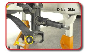
Remove the front spring & plate with a 1/2" Socket. Retain spring plate & hardware, discard spring.
