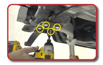
Attach the Tie Rod Mounts to the new Spindles using the supplied hardware as shown.
