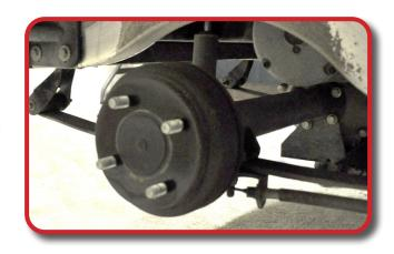
**NOTE:** It is highly recommended to use rear Heavy Duty Leaf Springs if installing a seat kit or cargo box on the rear of your golf cart. The shackle extensions will not be enough to support the weight and will cause too much stress on the single leaf factory spring.
