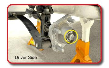
Using a 18mm Socket, remove the nut from the king bolt. Push shock/clevis up and out of the way.
