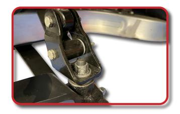
Attach the steering tie rod end to the new Spindle Mount and secure using retained factory nut and cotter pin.
