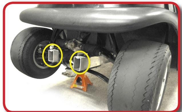
Using a 3/4" Socket remove front wheels.
