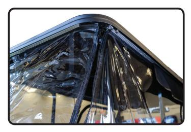
Using the Front Valance, slide it into the outside track. Pull until it is fully stretched. Repeat this process with the remaining valances around the entirety of the vehicle.
