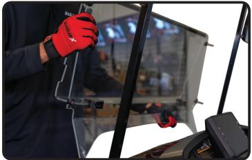
Wrap the front strut cover around the front struts and attach with the small zipper located on the inside.
