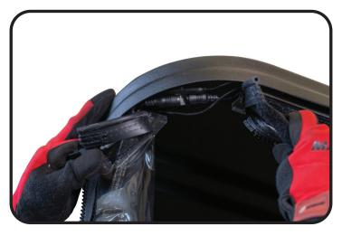
Now that all pieces are on the cart, ensure the enclosure and valances are properly aligned to match cart body lines. When satisfied, zip all corners of enclosure and attach all valance hook and loop strips.
