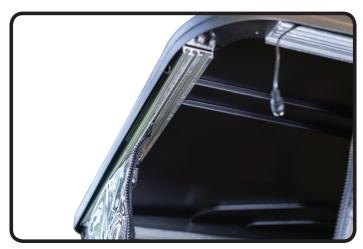
Next, with the camera wiring out of the way, feed the piping down the middle track. With hooks and storage straps on the inside pull the rear panel so it will connect with the zipper on the side panels, ensuring the cutout for the camera is centered. Connect and zip all the way down. The rear panel should go on outside of rear safety grab bar.
