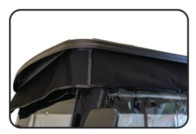
To install the rear valance slide it along the outside track. Pull until it is fully stretched and the camera cutout is centered with the enclosure cut out. You will then feed the camera cable through the wiring channel on the top of the versa top as shown and reconnect the camera cable. NOTE with the enclosure installed you will not be able to use the corner covers.
